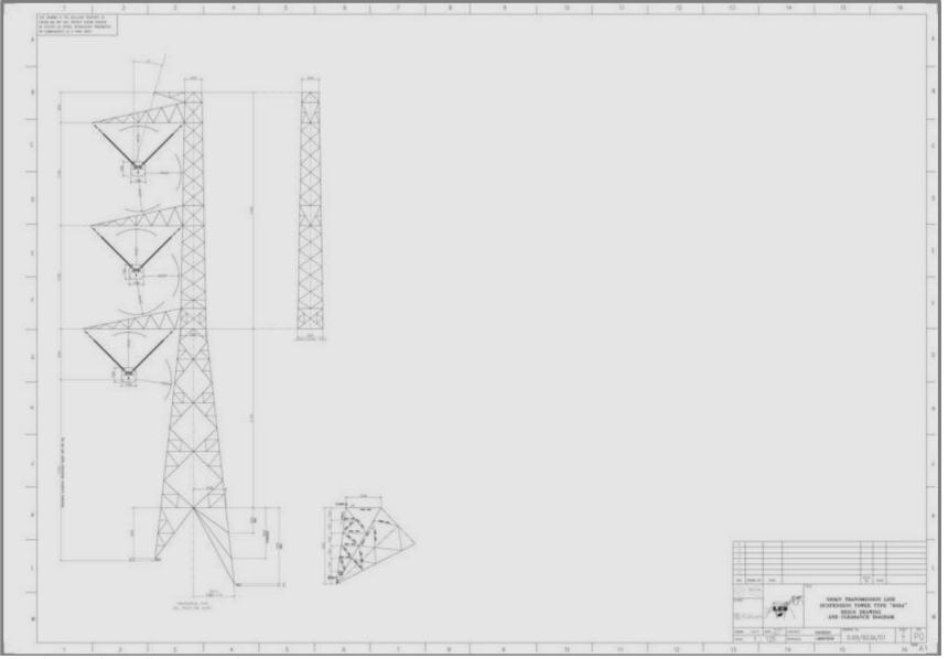
Figure 5: Proposed transmission line suspension tower
